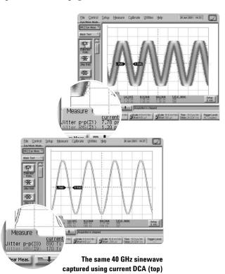
and now with 86107A precision timebase module (bottom).
